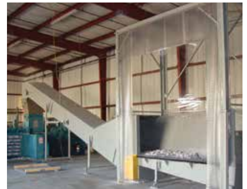
Dust Containment System, optional with all Allegheny Off-Loading Systems, minimizes dust produced from the off-loading process
