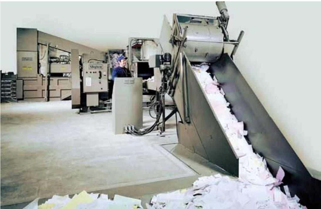
*Complete shredding system with automatic feeding system*
