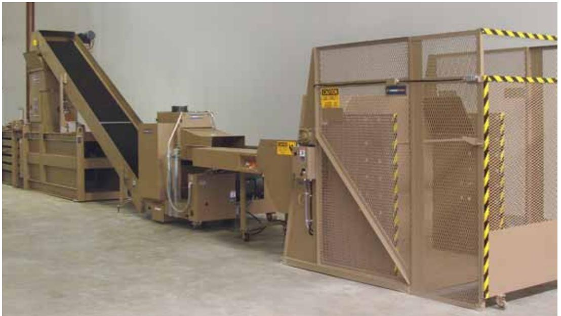
*A complete shredding system can include a tipper (or an automatic feeding system), paper shredder, output conveyor and baler*
