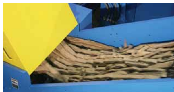
(above): Core being fed into the cutting assembly
