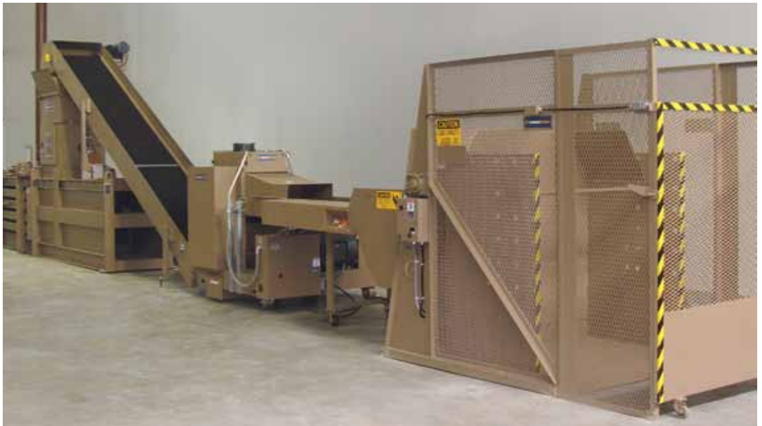
A complete shredding system can include a tipper (or an automatic feeding system), paper shredder, output conveyor and baler
