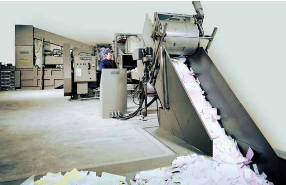
Complete shredding system with automatic feeding system
