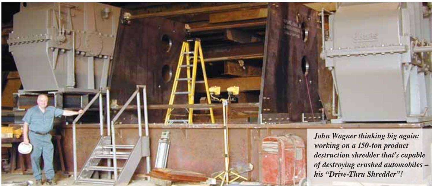
*John Wagner thinking big again: working on a 150-ton product destruction shredder that's capable of destroying crushed automobiles – his "Drive-Thru Shredder"!*
